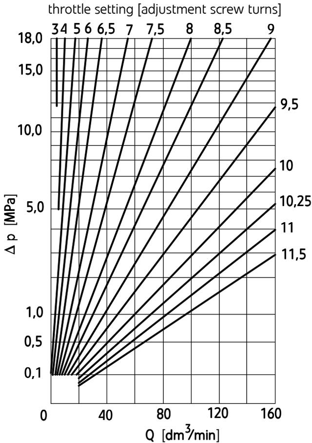
Flow resistance curves  $\Delta p(Q)$  for the check valve
