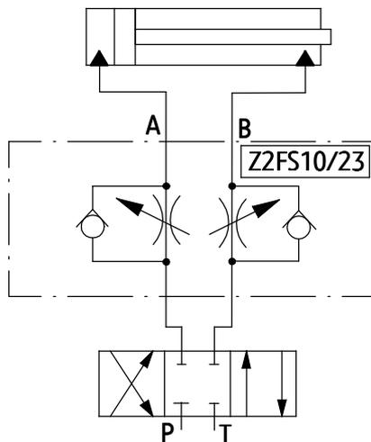
Flow throttling in the drain of the receiver (actuator) - valve fitted in rotated position by  $180^\circ$
